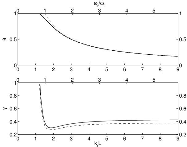
Figure 4: Comparison of the first regime for  $L=57\text{cm}$  (—) and  $L=14.69\text{cm}$  (---). Lower plot: dimensionless blowing pressure  $\gamma$  of the bifurcation. Upper plot: corresponding dimensionless frequency ratio  $\theta = \omega/\omega_r$ ; the first passive resonance of the bore is reminded ( $\cdots$ ).
