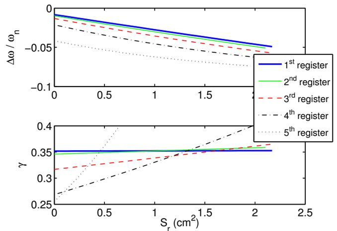
Figure 11: Variations of the oscillation threshold with respect to  $S_r$ : critical blowing pressure  $\gamma$  and relative frequency deviation from the bore resonances  $\Delta\omega/\omega_n$  for each of the five Hopf bifurcations. Parameters of the model:  $q_r = 0.3$ ,  $\zeta = 0.75$ ,  $f_r = 1500\text{Hz}$ .
