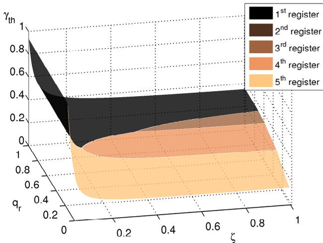
Figure 10: Oscillation threshold with respect to the reed damping parameter  $q_r$  and the control parameter  $\zeta$ . The blowing pressure threshold  $\gamma_{th}$  is calculated the same way as in figure 7-b. The surface shading indicate the selected regime.
