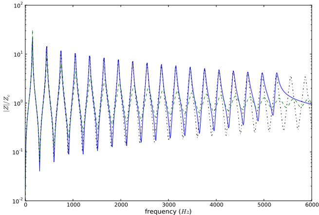
Figure 1: Impedance spectrum (reduced modulus) of a purely cylindrical bore of length  $L=57\text{cm}$  taking into account thermoviscous losses and radiation and truncated to 18 modes as used in this study (—), analytical impedance spectrum without modal decomposition (---), impedance spectrum used in Wilson and Beavers[9]. (-·-).
