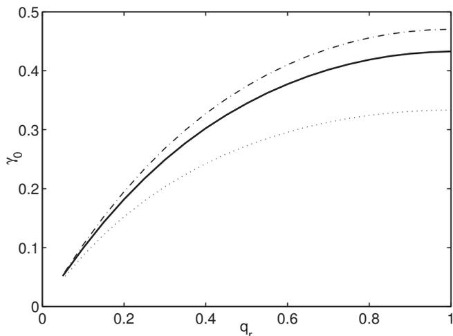
Figure 6: Minimum threshold  $\gamma_0$  as a function of  $q_r$ . Our numerical results (—), without approximation. Analytical results using two approximations: no loss ( $\cdots$ ), single-mode resonator with losses ( $- \cdot -$ ).
