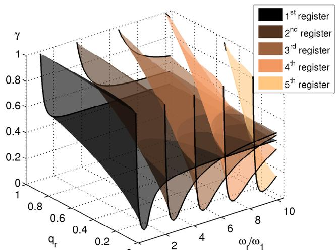
Figure 7: a) Similar plot as in figure 5 for the first five registers: the critical blowing pressure  $\gamma$  of each Hopf bifurcation is plotted with respect to the reed damping parameter  $q_r$  and frequency ratio  $\omega_r/\omega_1$ . The plain curves correspond to the smallest and highest  $q_r$  where a bifurcation occurs on the chosen range.
