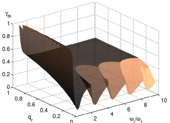
Figure 7: b) The oscillation threshold extracted from figure 7-a: blowing pressure at threshold  $\gamma_{th}$ , defined by the lowest of the five surfaces plotted in figure 7-a.
