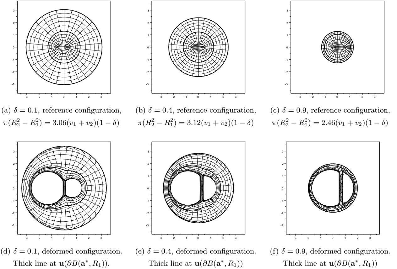
Figure 6: Transition to a radially symmetric map. A larger initial domain is necessary in order to create spherical cavities. Parameters:  $\Omega = B(\mathbf{0}, R_2)$ ,  $\sqrt{\frac{v_1 + v_2}{\pi d^2}} = 1.5$ ,  $\frac{v_2}{v_1} = 0.3$ ,  $d = 1$ ,  $R_1 \approx d$ .
