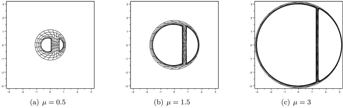
Figure 2: Incompressible deformation  $\mathbf{u} : B(\mathbf{0}, d) \setminus \{\mathbf{a}_1, \mathbf{a}_2\} \rightarrow \mathbb{R}^2$ ,  $d = |\mathbf{a}_2 - \mathbf{a}_1|$ , opening distorted cavities of volumes  $v_1 + \pi\varepsilon_1^2$ ,  $v_2 + \pi\varepsilon_2^2$ ; deformed configuration for increasing values of the displacement load ( $\mu := \sqrt{\frac{v_1 + v_2}{\pi d^2}}$ ). Choice of parameters:  $d = 1$ ,  $\frac{v_2}{v_1} = 0.3$ .
