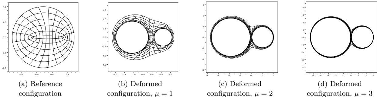
Figure 3: Incompressible deformation of  $B(\mathbf{0}, d)$ ,  $d := |\mathbf{a}_2 - \mathbf{a}_1|$ , for increasing values of  $\mu := \sqrt{\frac{v_1 + v_2}{\pi d^2}}$ . Final cavity volumes  $v_1$  and  $v_2$  given by  $d = 1$ ,  $\frac{v_2}{v_1} = 0.3$ .
