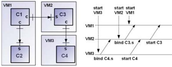
Figure 2. Application configuration (left) and self-configuration protocol (right)
