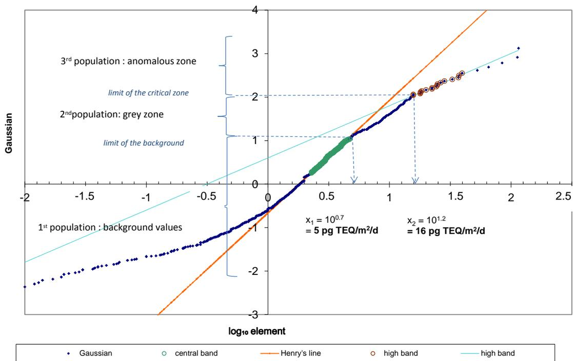
Figure 2 – TEQ deposition data treatment: graphical representation of Henry's line method<sup>5,6,7</sup>.
