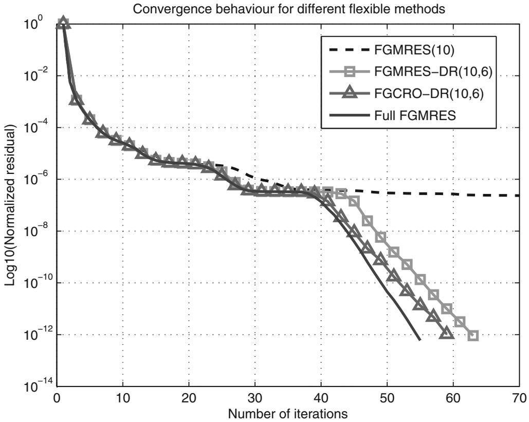
FIG. 3.1. Convergence histories of different flexible methods applied to  $Ax = b$ , where  $A \in \mathbb{R}^{200 \times 200}$  is symmetric positive definite with some eigenvalues of small magnitude.
