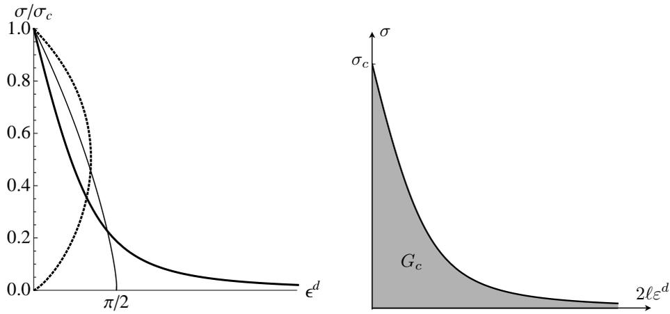
**Fig. 7** Left: evolution of  $\varepsilon^d$  (part of the average strain of the bar due to damage in a localization zone) in a stress-strain diagram. Here are plotted the curves associated with three models of Example 1. Dashed line:  $p = 0.5$ ,  $q = 1$ ; thin line:  $p = 1$ ,  $q = 2$ ; thick line:  $p = 2$ ,  $q = 4$ . Right : graphical identification of the fracture energy
