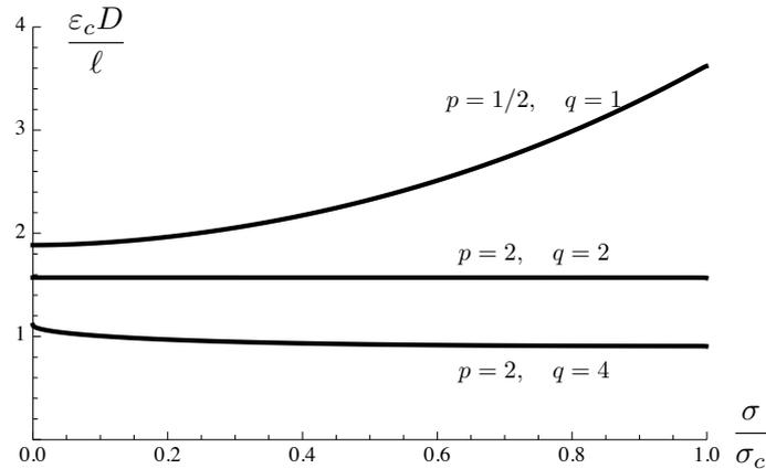
**Fig. 4** Evolution of the half-length of the damage zone as a function of the stress for three models of the family of brittle materials of Example 1: for  $p = 1/2$  and  $q = 2$ ,  $D$  decreases all along the damage process; for  $p = q = 2$ ,  $D$  remains constant; for  $p = 2$  and  $q = 4$ ,  $D$  increases all along the damage process.
