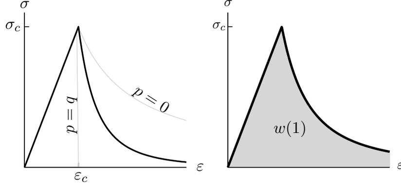
**Fig. 1** Left: The stress-strain response (black curve) associated with the homogeneous evolution in the case of the models of Example 1 with  $q > p > 0$ . The limit cases of perfectly brittle material ( $p = q$ ) and weakly brittle material ( $p = 0$ ) are in gray. Right: Graphical interpretation of the dissipated energy at the end of a homogeneous damage process.
