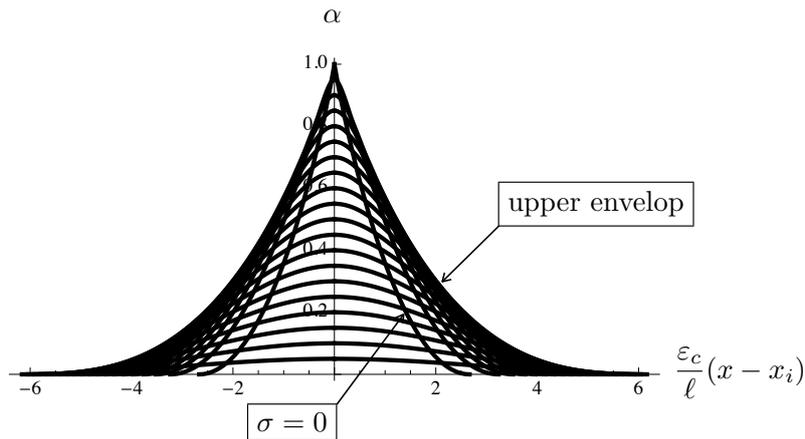
**Fig. 6** Construction of an evolution which respects the irreversibility condition in the case where the size of the damage zone predicted by the initial construction decreases while the stress decreases. This consists in taking the upper envelope of the evolution obtained without the irreversibility condition. Here is the case when  $p = q = 1/2$ . Note the gap between the upper envelope and the previously considered damage profile when the bar breaks.
