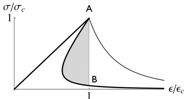
**Fig. 10** Case of a long bar ( $L > L_s$ ). Because of the snap-back of the response with lowest energy and the instability of the homogeneous response (thin curve), the evolution is discontinuous at the bifurcation point A. If the state of the bar jumps from A to B then the energy corresponding to the gray area is transformed into kinetic energy or into energy dissipated in further damage.
