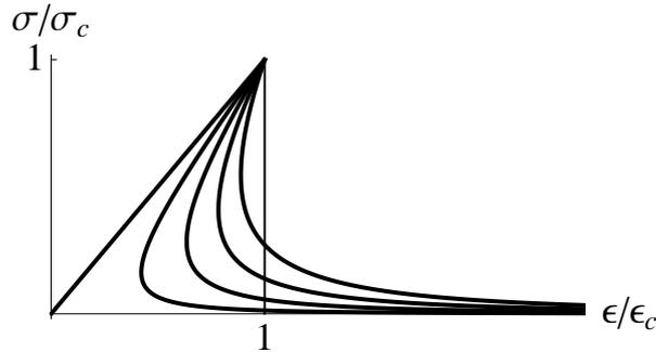
**Fig. 9** Overall stress-strain responses for the model of Example 1 with  $p = q = 4$  (hence  $D_0 = 1.67D_c$ ). Thin curve: homogeneous response; Thick curves: responses with localization of damage after the elastic phase. For  $L > D_c$  (here  $L = 4D_0 \approx 6.67D_c$ ), half localization zones can appear (here up to 6, but only the first four are plotted), all present a snap-back and go to infinity. The lowest curve corresponds to  $i = 1$ .
