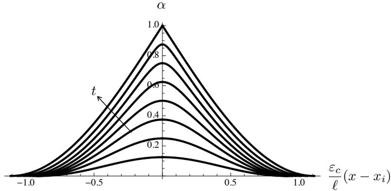
**Fig. 5** The damage profile for a given  $t$  and its evolution with  $t$  by assuming that  $t \mapsto \sigma_t$  is decreasing in the case of the model of Example 1 with  $p = 2$  and  $q = 4$ . The rupture occurs when  $\sigma_t = 0$  and  $\bar{\alpha}(\sigma_t) = 1$ . We check numerically that  $\sigma \mapsto D(\sigma)$  is decreasing, see Figure 4.
