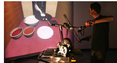
Figure 2: Setup: Bimanual interaction with two 6-DoF haptic devices (Virtuose, Haption). Left hand for virtual bowl manipulation, Right hand for virtual pan manipulation.
