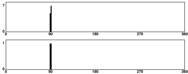
Figure 22: Top: histogram of angles between chained line segments corresponding to the image of figure 2. Bottom: meaningful histogram mode detected.
