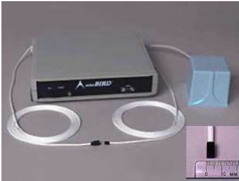
Fig. 12. MiniBIRD 6 DOF magnetic sensor
