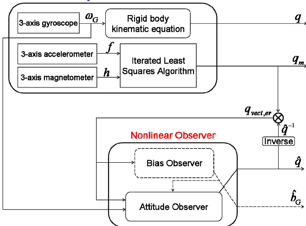
**Fig. 2.** Block diagram for the attitude and bias estimation algorithm
