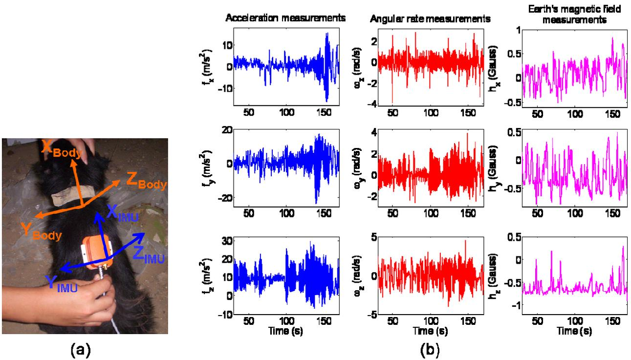
Fig. 5. (a) The MTi-G attached to the back of the dog – (b) Acceleration, angular rate and magnetic field measurements from the MTi-G during the motion of the dog
