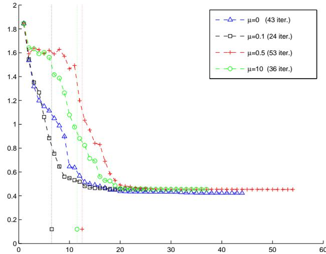
FIG. 7.2. Full order mixed  $H_2/H_\infty$  synthesis for the four disks problem: the values of the  $H_2$  norm in relation to the number of serious steps are shown for four different values of the penalty parameter  $\mu$ . Here we choose:  $\mu \in \{0, 0.1, 0.5, 10\}$ . Vertical lines point out the instant at which the iterates become feasible.
