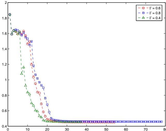
FIG. 7.3. Full order mixed  $H_2/H_\infty$  synthesis for the four disks problem: the values of the  $H_2$  norm versus the number of serious steps for three different values of the parameter  $\Gamma \in \{0.4, 0.6, 0.8\}$ .
