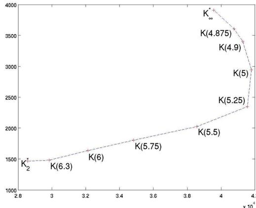
FIG. 7.1.  $H_2/H_\infty$  optimal static controllers  $K(\gamma_\infty) = (K_1(\gamma_\infty), K_2(\gamma_\infty)) \in \mathbb{R}^2$  for the vehicular suspension control problem.  $[\|T_\infty(K_\infty)\|_\infty, \|T_\infty(K_2)\|_\infty] \ni \gamma_\infty \mapsto K(\gamma_\infty)$  continuously transforms the  $H_\infty$  optimal gain  $K_\infty$  into the  $H_2$  optimal gain  $K_2$ .
