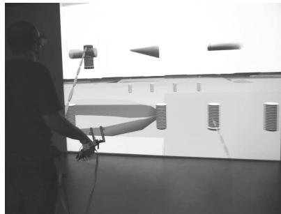
Figure 4: An immersive musical environment with four 3D reactive widgets , three tunnels and Piivert (first prototype). Four other widgets can be seen further in the environment.
