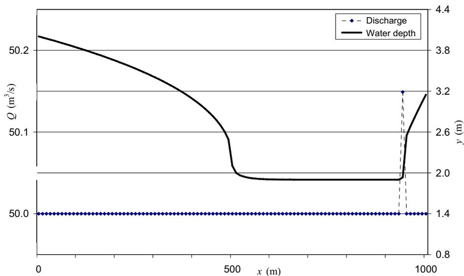
Figure 8 Profile of  $Q(x)$  at intermediate steady state
