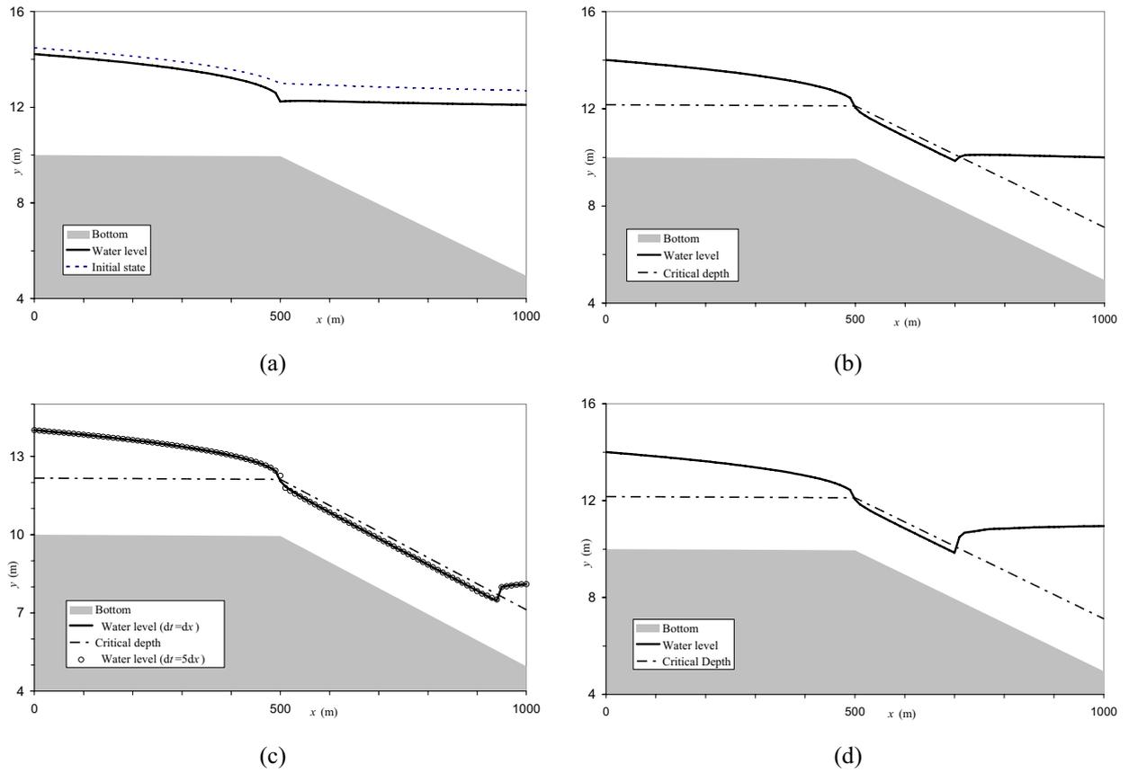
Figure 6 Solution evolution with (a) Appearance of the transcritical zone, (b) Downstream moving shock, (c) Intermediate steady state with  $dt=dx$  and  $dt=5dx$ , (d) Upstream moving shock
