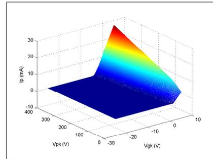
Fig. 2: Characterization surface for the  $I_p$  current
