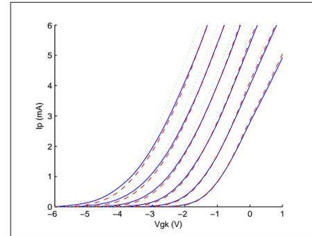
**Fig. 3:** Interpolated currents from the triode (1), the triode (2), and the triode (3)
