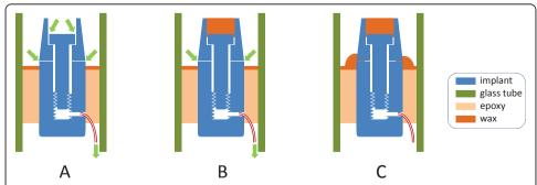
**Figure 3 Test conditions applied**. Test conditions applied for each implant (green arrows indicate the possible leakage paths): A) abutment manual screwing. Nitrogen flow may occur at both gaps: between screw and abutment and between abutment and implant collar (assay 1). B) screw hole blocked with wax; manual (assay 2) or key (assay 3) screwing. C) abutment key screwing, screw hole and implant to abutment connection blocked with wax (as a negative test).
