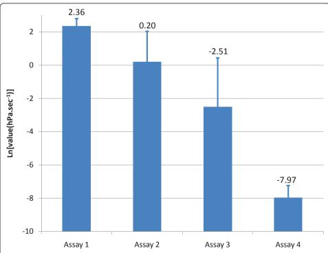
**Figure 5 Gas leaking in four conditions**. Gas leaking for the tested implants (values are indicated up bars):Assay 1, abutment manual screwing; Assay 2, abutment manual screwing, screw hole blocked with wax;Assay 3, abutment key screwing, screw hole blocked with wax; Assay 4, negative test with abutment key screwing, both screw hole and implant to abutment connection blocked with wax.
