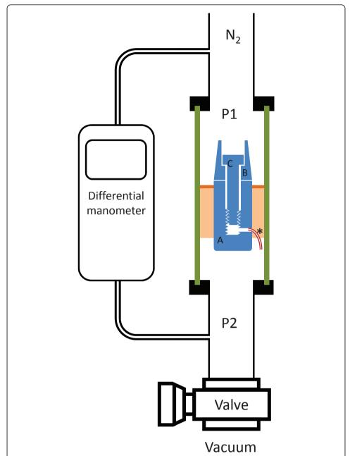
**Figure 1 Experimental set-up.** Nitrogen leaks from chamber P1 to chamber P2 through the gap between implant (A) and abutment (B) and between the screw (C) and the abutment, then through a plastic tube (\*) connecting the internal chamber of the implant with chamber P2. In the glass tube (green), the implant is sealed in epoxy adhesive (pink) and the tightness is ensured with wax (brown).
