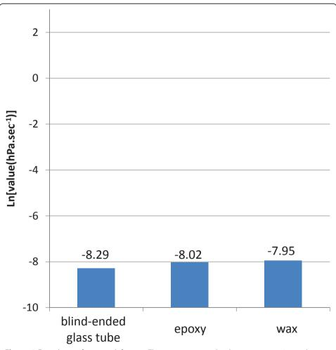
**Figure 4 Experimental set-up tightness.** Three tests were realized to assess experimental set-up tightness: -blind-ended glass tube; - epoxy: a double-ended opened glass tube sealed on one side with a plug of epoxy glue;- wax: a double-ended opened glass tube sealed on one side with a plug of wax.
