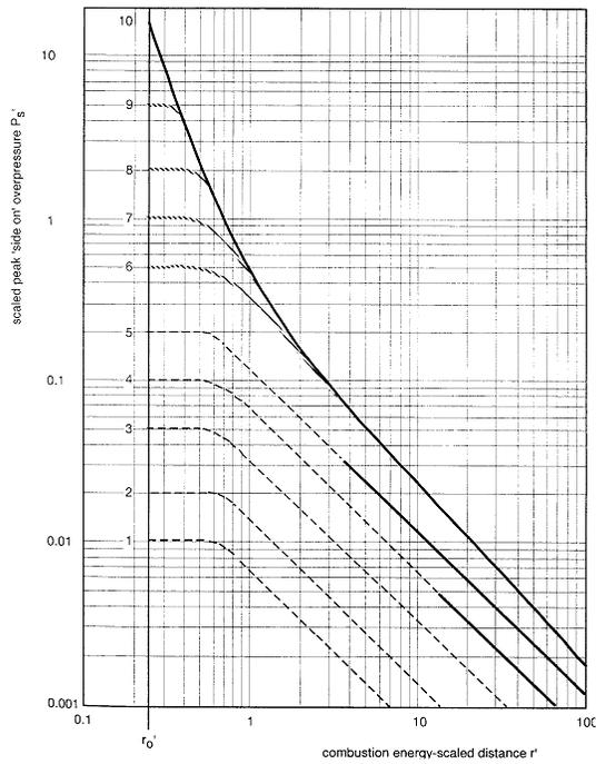
Fig. 5. Reduced pressure - TNO type multi-energy method (CPR, 1997)
