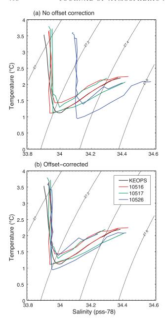
FIG. 7. Superposition of a selection of T/S diagrams taken in the same area (51°S, 75°E) from CTD–SRDLs 10516 (red), 10517 (green), and 10526 (blue). A close historical profile from the KEOPS cruise (see Park et al. 2008) is also overlaid (black). The profiles are shown (a) before and (b) after the salinity offset correction.
