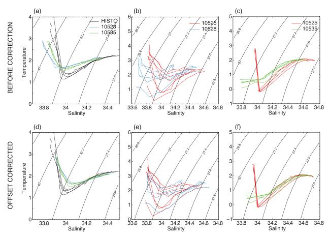
FIG. 8. Comparisons of close *T/S* diagrams from CTD–SRDLs 10525, 10528, and 10535 in 3 different locations. In each cases, and although these comparisons are done far from the Northern Kerguelen Plateau, the *T/S* diagram overlapping is improved after the offset correction.
