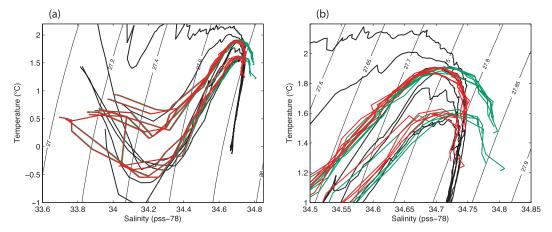
FIG. 5. Comparison between several selected profiles of the CTD–SRDL 10516 and historical profiles. Selected CTD–SRDL profiles are presented with no correction (green) and after the pressure-effect correction (red). Close historical profiles with comparable *T/S* properties are overlaid (black). (a) The *T/S* curves and (b) zoomed on their deep part. The pressure-effect correction allows a much better overlapping with historical *T/S* diagrams at depth.
