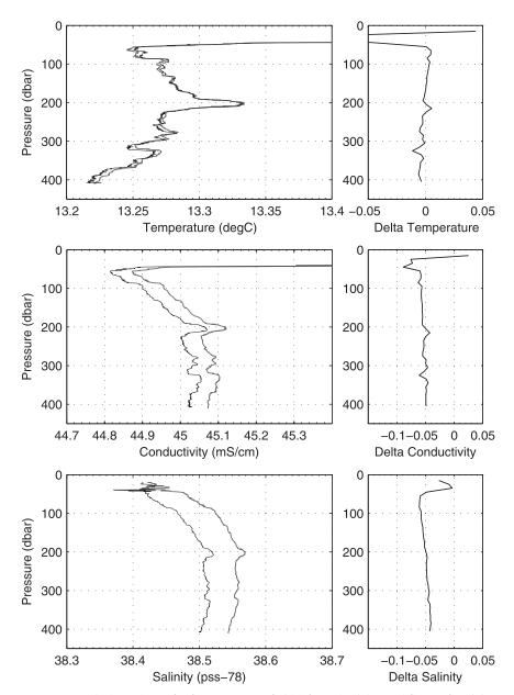
FIG. 3. Vertical profiles of (top) temperature, (middle) conductivity, and (bottom) salinity sampled by CTD–SRDL 10516 (black) and the ship-based CTD (gray) during the same cast. (right) Differences between the CTD–SRDL and the SBE25.
