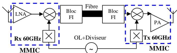
Figure 2. Architecture Tx/Rx
