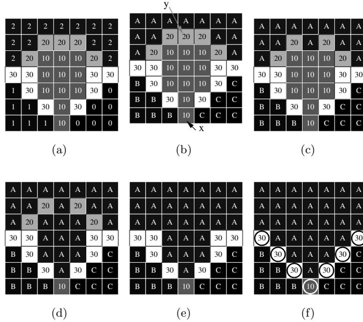
**Fig. 2.** (a): Original image. (b-f): several steps of the flooding algorithm. One can see that this algorithm is not “monotone”: some points at altitude 10 are processed after one of the points at altitude 20. One can also note that the contour at altitude 20 in the original image (a) is not present in the result (f).
