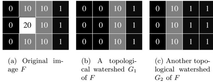
**Fig. 10.** An image (a), and two associated topological watersheds (b) and (c). Note that, contrary to the topological watershed (b), the topological watershed (c) cannot be obtained through a reverse W-flooding process.
