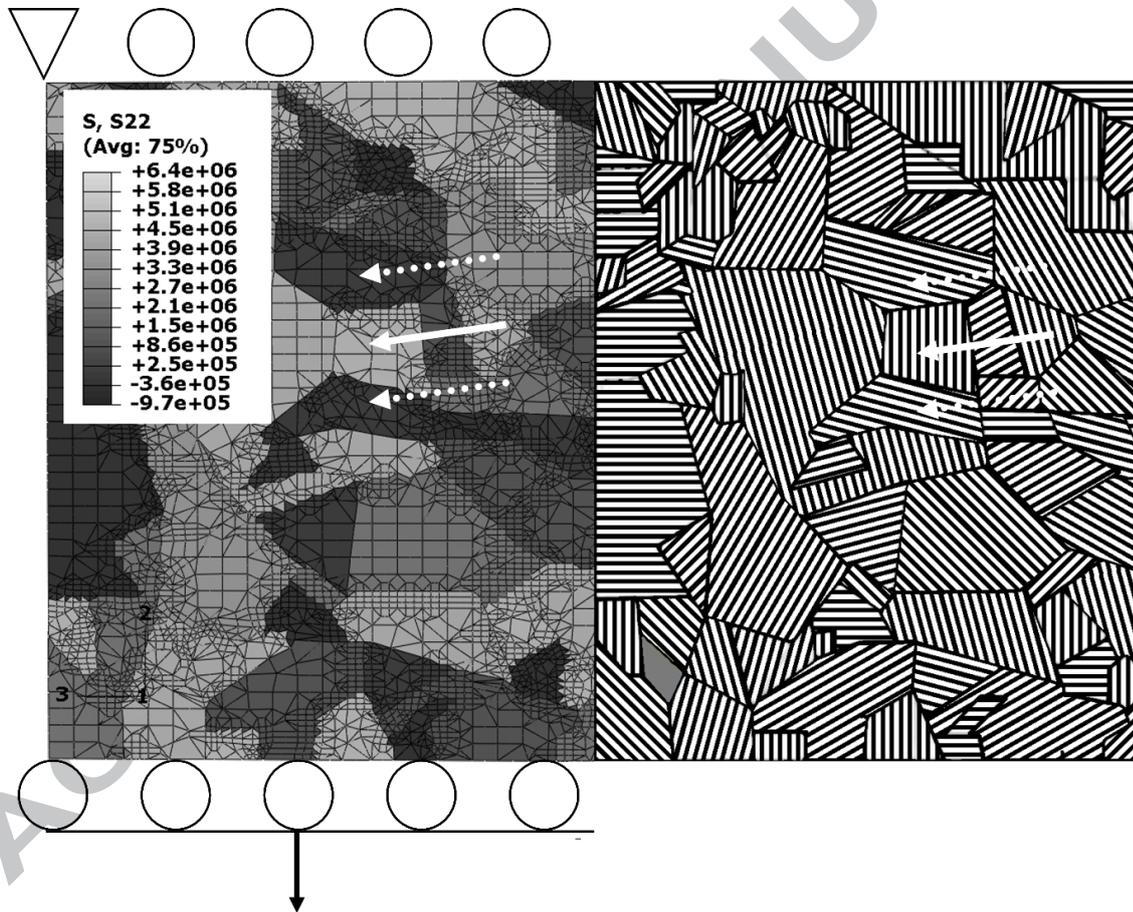
Figure 9: left: Detail of the  $\sigma_{22}$  (in Pa) stress distribution in the microstructure for a vertical load (along the 2-direction) in the mesoscopic model for 39 % ceramic content. Right: shape and orientation of the domains in the polydomain specimen modelled on the left. The solid white arrows indicate a domain with high stresses and lamellae oriented along the loading
