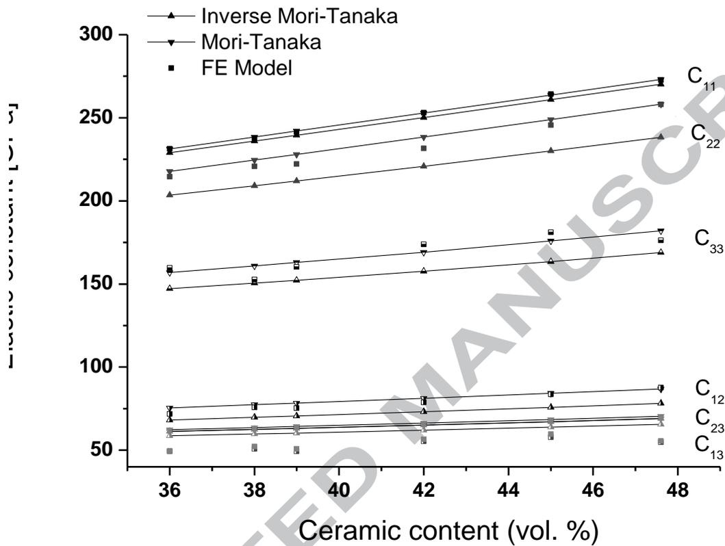
Figure 5: Elastic constants for single domain samples with different ceramic contents.  $C_{11}$ ,  $C_{22}$  and  $C_{33}$  are the diagonal elements of the stiffness matrices and  $C_{12}$ ,  $C_{13}$  and  $C_{23}$  are the constants for shearing. Results of FEM-calculations and estimations using Mori-Tanaka and inverse Mori-Tanaka models are presented as squares and triangles.
