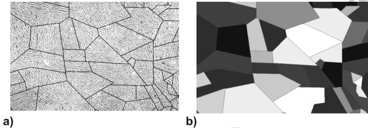
Figure 2: a) Micrograph of a typical polydomain specimen divided into domains of parallel lamellae orientation; b) Each domain was filled with a colour according to the domain orientation angle  $\alpha$ .
