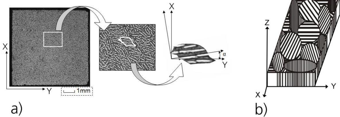
Figure 1: **a)** Polarised light microscopy micrograph of the microstructure and single domain with orientation  $\alpha$  to global coordinate system, **b)** Axis convention for a schematic presented polydomain freeze-cast MMC (specimen size 8 x 60 x 40 mm<sup>3</sup>) used in this study. Z denotes the freezing direction with parallel lamellae; X is the direction of the long side and Y the direction of the short side of the specimen.
