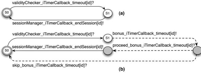
Fig. 8. ValidityChecker template adaptation (a) original, (b) adapted
