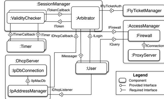
Fig. 1. Architecture of the airport internet access system
