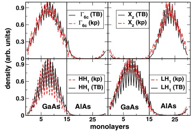
FIG. 3. (Color online) Hole and electron wave functions of the  $(\text{GaAs})_{15}/(\text{AlAs})_{15}$  SL obtained with the 30-band  $\mathbf{k}\cdot\mathbf{p}$  (dash lines) and TB (full lines) models.
