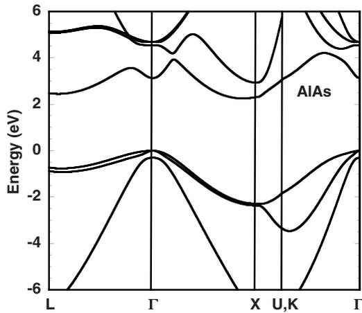
FIG. 1. Electronic band structure of bulk AlAs calculated with the 30-band  $\mathbf{k}\cdot\mathbf{p}$  model at  $T=0$  K. The model parameters are given in Table I and some values of the band energies and effective masses in Table II.
