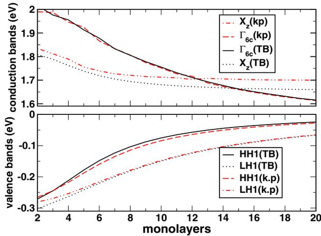
FIG. 2. (Color online) Comparison of the near-band gap energies of the  $(\text{GaAs})_n/(\text{AlAs})_n$  SL at the zone center of the BZ as function of period  $n$ . Full and dot lines correspond to TB results, while dash and dash-dot lines correspond to  $\mathbf{k}\cdot\mathbf{p}$  results. The energy zero is taken at the bulk GaAs valence band maximum.
