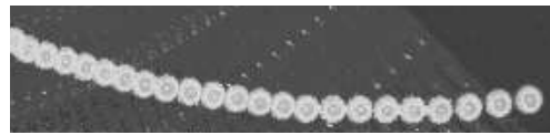
FIGURE 2: Typical sequence showing the spinning motion of a spherical particle onto the rotating plate.
