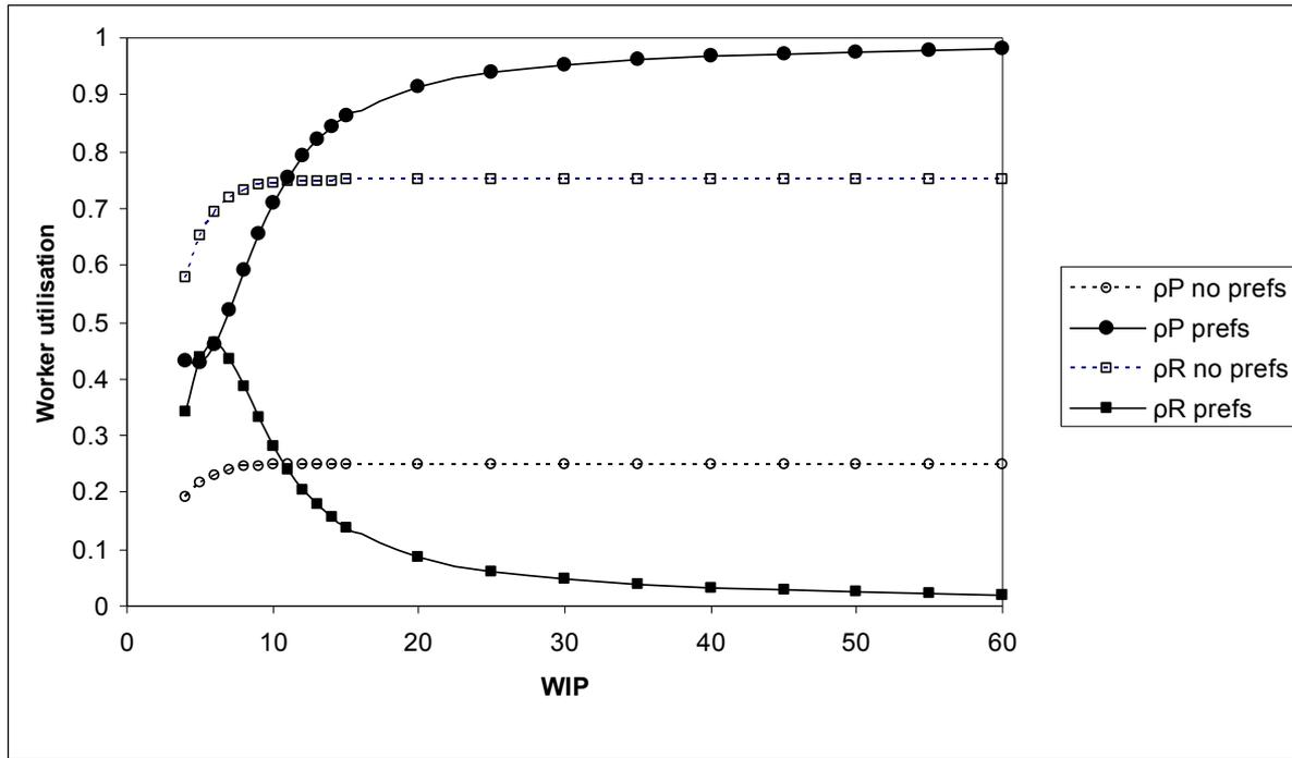
Figure 7 Utilisation of workers from their preferred machines ( $\rho P$ ) and remaining machines ( $\rho R$ ) with and without worker preferences for the full flexibility configuration.
