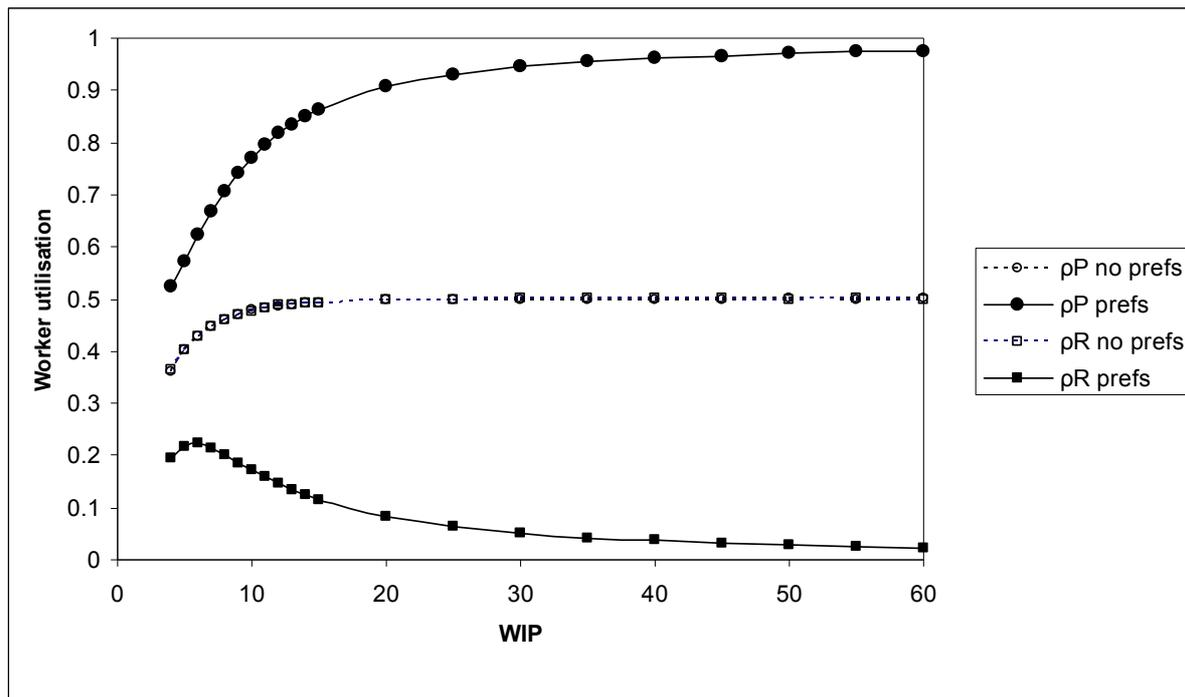
Figure 6 Utilisation of workers from their preferred machines ( $\rho P$ ) and remaining machines ( $\rho R$ ) with and without worker preferences for the 4-skill chaining configuration.
