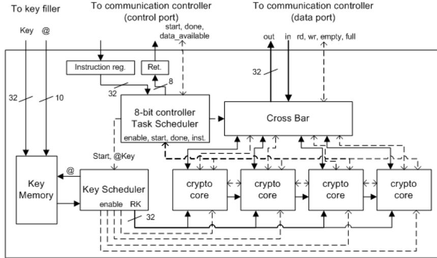
Fig. 1. The M CCP Architecture
