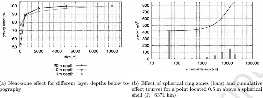
Figure 1: Contribution of zones of different size to the gravitational effect induced by a water layer of 1 m thickness.
