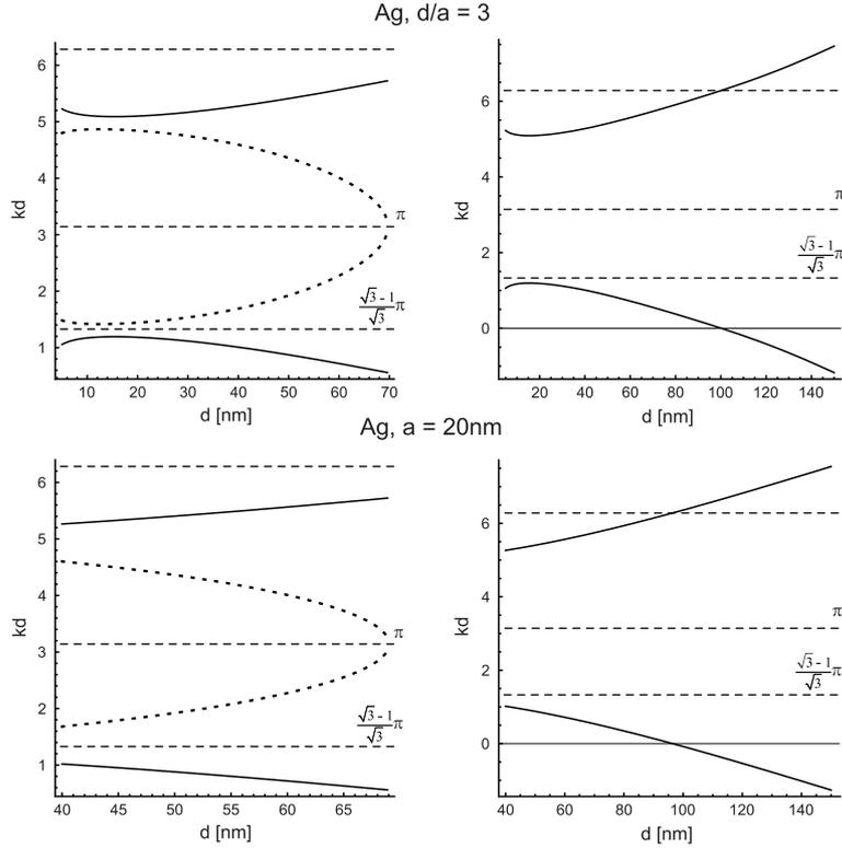
**Figure 3.** Wave vector  $kd$  for undamped surface plasmon propagation along the metallic nano-sphere chain versus sphere separation  $d$  at (top) constant  $d/a = 3$ , with  $a$  the sphere radius, and (bottom) for  $a = 20$  nm for Ag sphere chains, respectively; transversal modes are shown by solid lines, while longitudinal modes are shown by dotted lines
