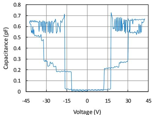
Fig. 5. Measured capacitance versus voltage for 60-GHz MEMS.
