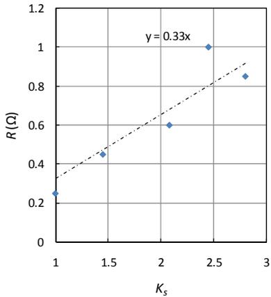
Fig. 10. Series resistance versus  $K_s$ .
