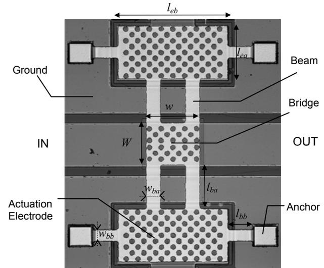
Fig. 2. Microphotograph of the fabricated reference switch.
