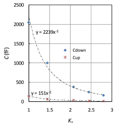
Fig. 8. Capacitance in up-state and down-state versus  $K_s$ .
