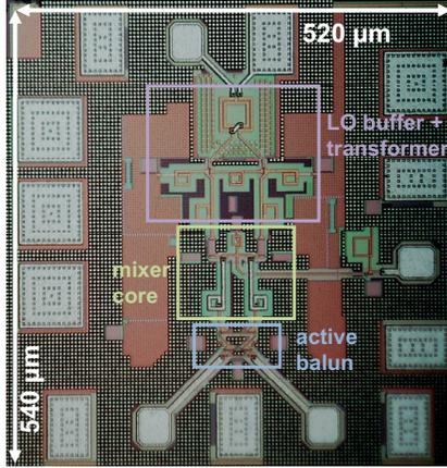
Figure 4: Die photograph of mixer circuit, size pad-limited
