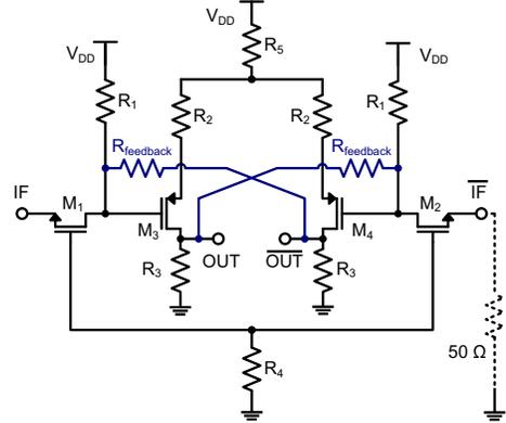
Figure 3: Simplified schematic of the IF buffer / active balun
