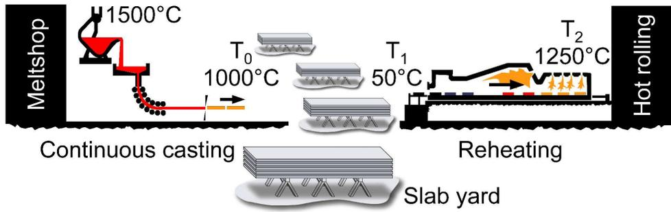
Steel production with continuous casting, reheating and hot rolling. The slab yard serves as buffer and inventory.
