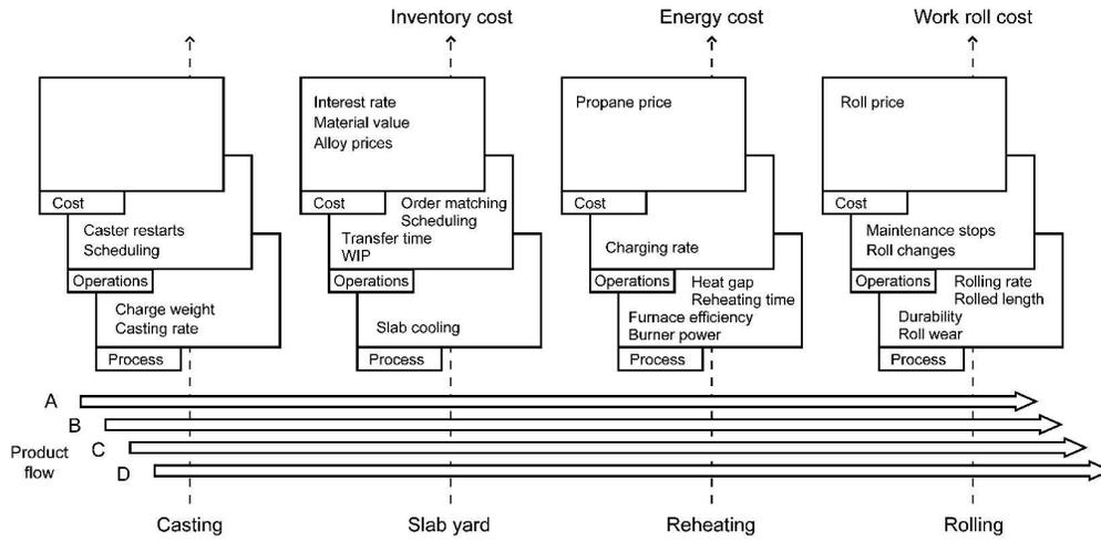
The three-layered cost model with processes, operations and cost components. The del contains four parallel product flows.
