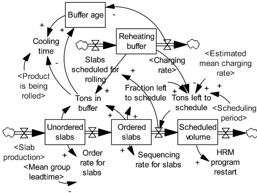
The interface between continuous casting and hot rolling, with order matching and scheduling.
