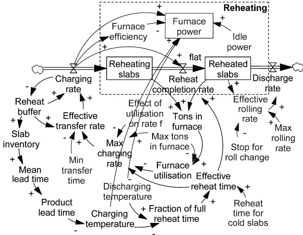
Reheating modelled as a two step process.
