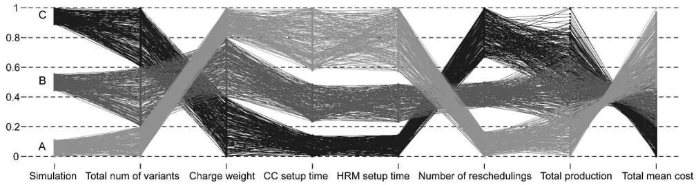
Parallel coordinate plot showing design parameters and simulated performance in terms of total mean cost and production volume for current (A) and future (B, C) plant configurations according to Table 1.
