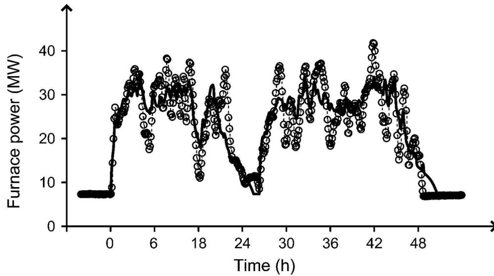
Validation of simulated furnace power (solid) against plant data (-o-). Charging and discharging rates in the model were based on smoothed data from the production database.
