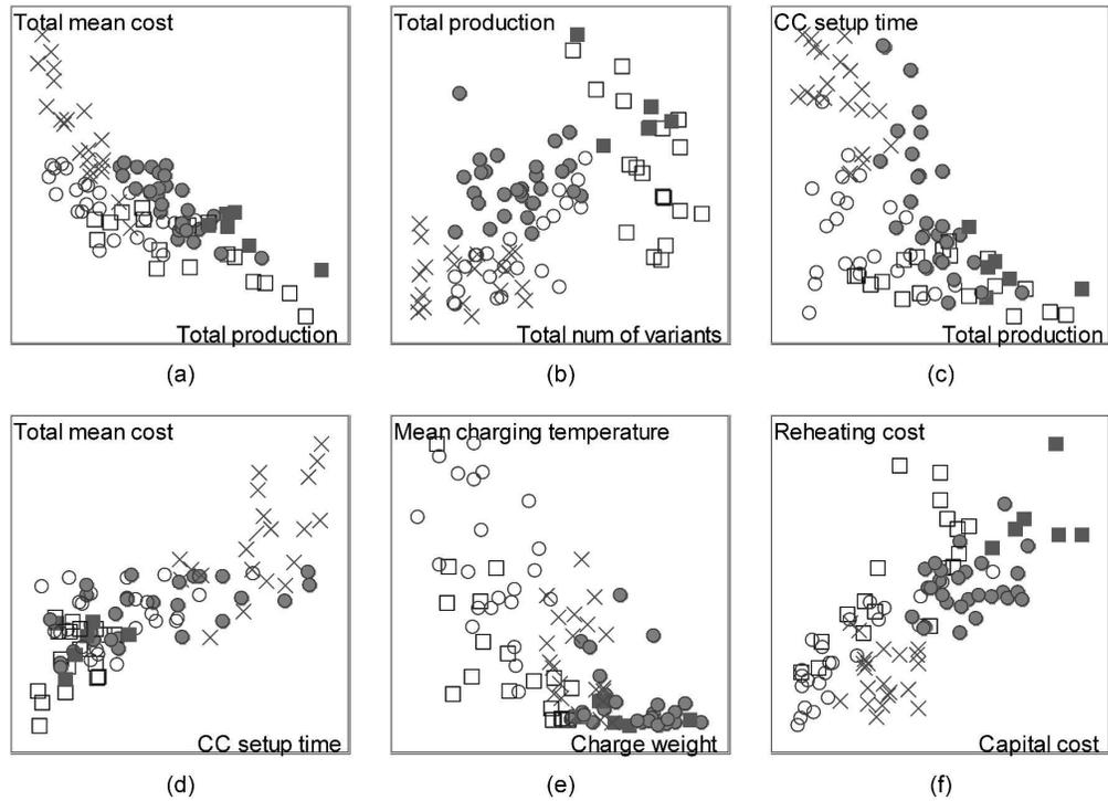
Exploring simulation results for configurations that combine increased product range with low cost. Current configuration indicated by (x). Configurations satisfying first goal with increased charge weights indicated by (●), and with reduced charge weights (○). Second goal with increased charge weights (■), and with reduced charge weights (□).
