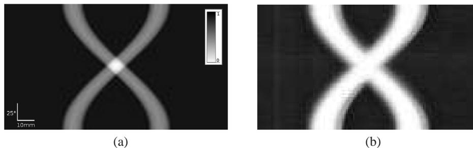
Fig. 3. Sinograms of two metallic bars (12 mm diameter) separated by 50 mm, with a projection number  $N_\theta = 72$ . (a) Ideal theoretical sinogram calculated by direct Radon transformation of a synthetic model. (b) Acquisition using the millimeter wave tomographic scanner with the 110 GHz source. Same scale and range as in (a).
