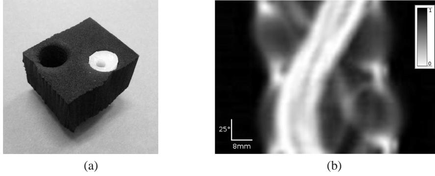
Fig. 2. (a) Photograph of original object: parallelepiped black foam ( $41 \times 49$ ) mm<sup>2</sup> with 2 holes, diameter 15 mm (1 hole with air and 1 hole containing a Teflon cylinder with a 6 mm cylindrical air hole inside). (b) Sinogram with  $N_\theta = 72$  projections (lines) and  $N_\rho = 128$  samples per projection (columns). Acquisition with the 110 GHz source.
