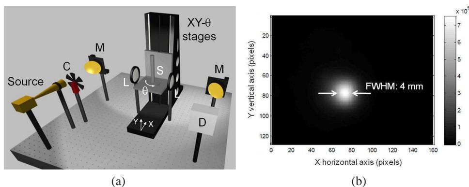
Fig. 1. (a) Experimental setup. C: optical chopper, L: Teflon lens ( $f' = 60$  mm), M: off-axis parabolic mirror ( $f' = 150$  mm), S: sample, D: pyroelectric detector. (b) 2D spatial profile of the THz beam waist at the sample position (110 GHz source) visualized with a photothermal THz converter (Teracam).
