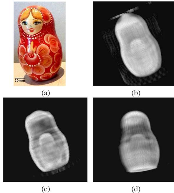
Fig. 9. Wooden Russian doll *Matriochka* (total height 160 mm). (a) Photograph of the 3D sample. (b) BFP reconstruction (Media 4). (c) SART reconstruction (Media 5). (d) OSEM reconstruction (Media 6). Acquisition with the 110 GHz source.
