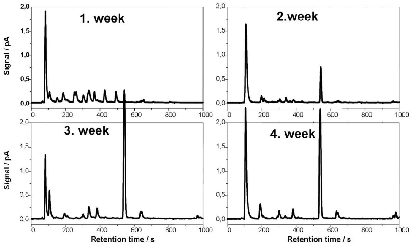
**Figure 3.** The growth of a mold culture leads to changes of the composition of the metabolites. The resulting IMS chromatogram (GC-UV-IMS) can be used to characterise the state of the culture.
