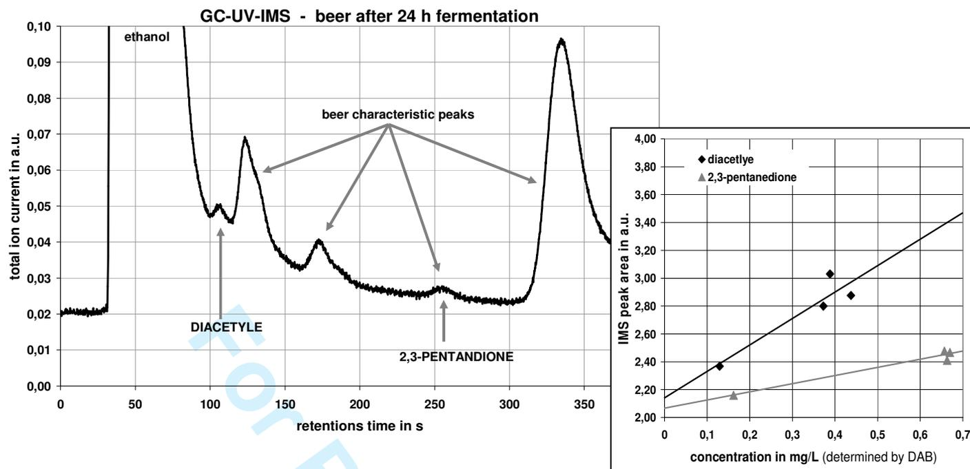
**Figure 2.** GC-UV-IMS chromatogram of beer (left) – the relevant diacetylye and 2,3-pentandione signals are indicated. Comparison (right) of the IMS signal peak area and the breweries routine measurements of diacetylye and pentandione for different fermentation duration.
