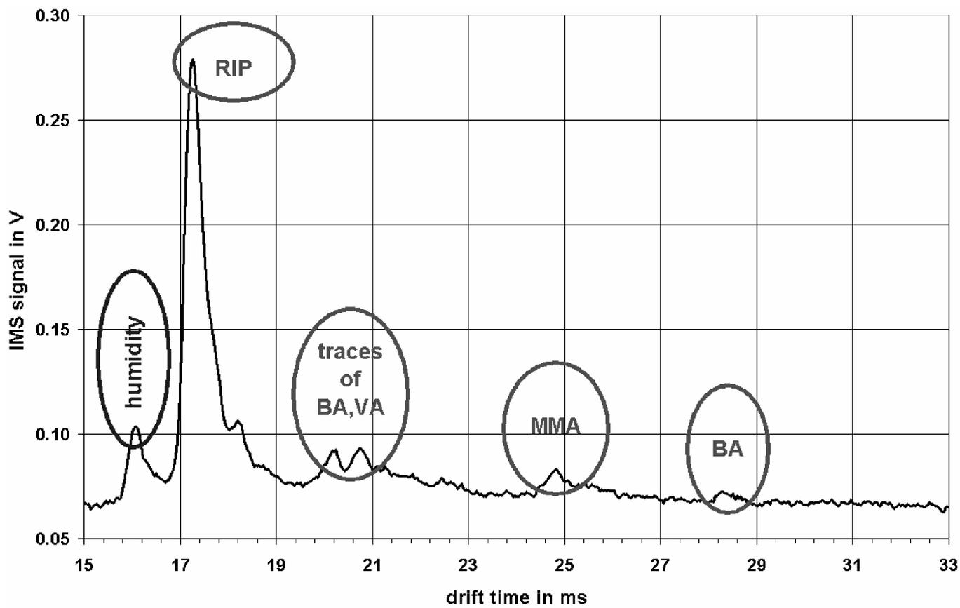
**Figure 6.** Traces of the initial monomers can be detected in the final polymer even after complete polymerisation.
