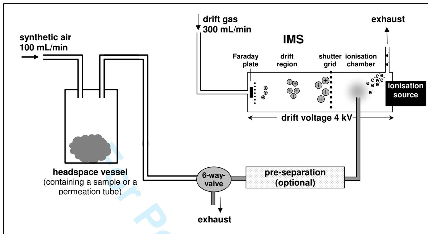
**Figure 1.** Scheme of an ion mobility spectrometer including pre-separation and headspace sampling unit.
