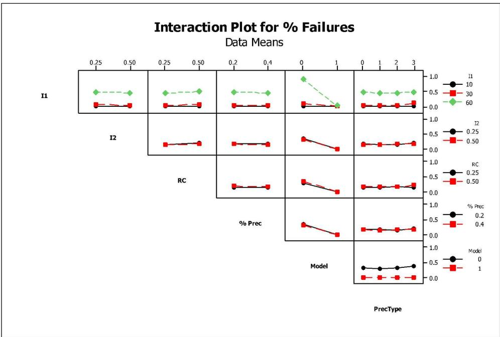
Figure 8. Interaction Plot for mean failures percentage.
