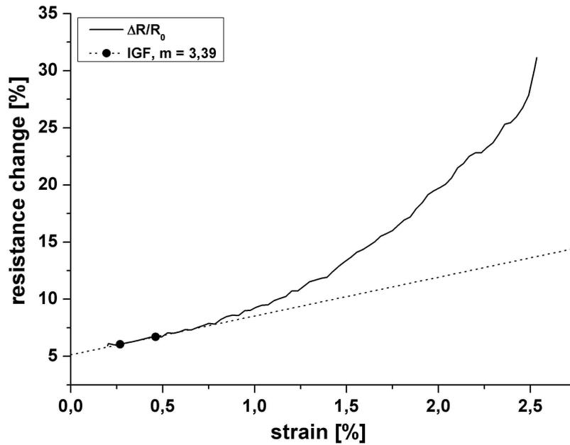
**Figure 7:** Electrical resistance change vs. mechanical strain, measured during the 10<sup>th</sup> loading cycle of a cyclic tensile test (resistivity measured in z-direction) for **a)** the composite containing 0.3 wt.% of MWCNTs and **b)** the composite containing 0.3 wt.% of carbon black.
