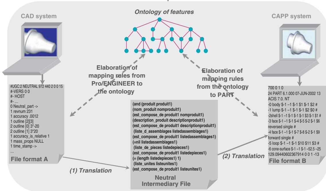
Figure 1. Global process for data exchange using ontologies.
