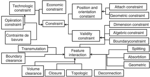
Figure 5. Constraint classification.
