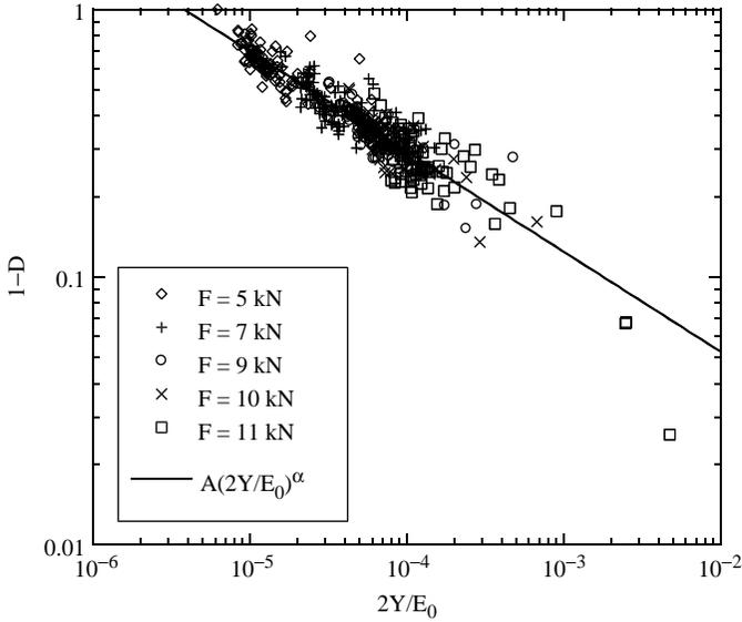
**Figure 6.** Change of  $1-D$  after correction with  $2Y/E_0$  when all load levels are considered and only the thermodynamically admissible data are kept. The symbols are identification points and the solid line is the best fit according to Equation (33).
