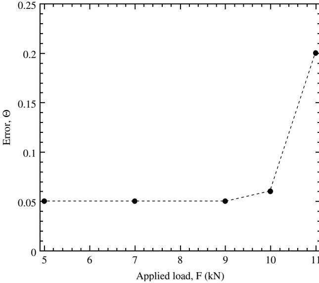
**Figure 3.** Error indicator  $\Theta$  vs load level. From the analysis of the results, it is expected that crack initiation occurred between 9 and 10 kN.
