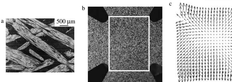
**Figure 1.** (a) Microstructure of the studied composite; (b) view of the sample and region of interest (white box); and (c) displacement field measured by digital image correlation for one load level (11 kN) close to failure (11.1 kN) in the region of interest.
