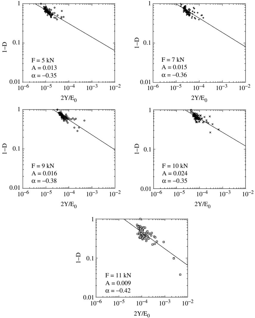
**Figure 4.** Change of  $1-D$  with  $2Y/E_0$  for five different load levels. The symbols are identification points and the solid line is the best fit according to Equation (33). The values of the identified parameters are reported for each load level. For the sake of comparison, the same range is used for all load levels.
