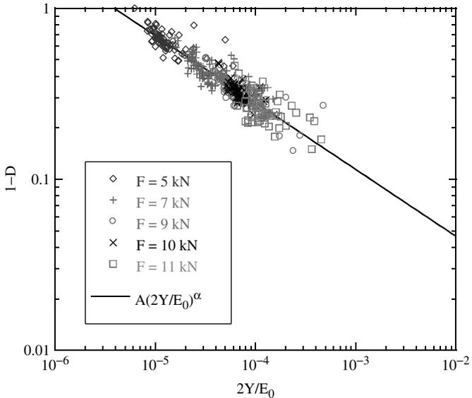
**Figure 7.** Change of  $1-D$  after correction with  $2Y/E_0$  when all load levels are considered. The thermodynamic consistency and identification accuracy are enforced. The symbols are identification points and the solid line is the best fit according to Equation (33).
