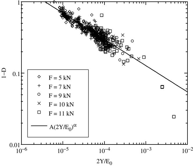
**Figure 5.** Change of  $1-D$  after correction with  $2Y/E_0$  when all load levels are considered in one identification so that a single value for the power  $\alpha$  is obtained. The symbols are identification points and the solid line is the best fit according to Equation (33).
