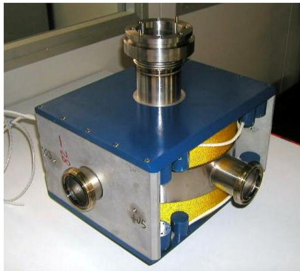
Fig. 1. Photo of the 8 T superconducting magnet with its radial access ports before the installation.
