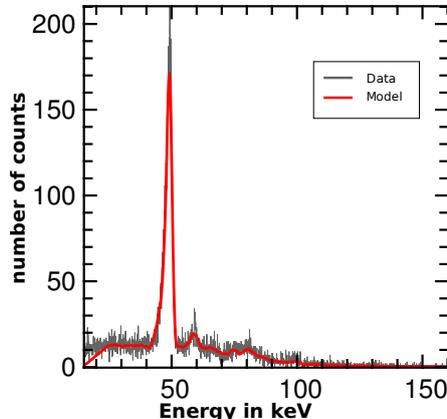
Figure 2: *Scattering measurements on a Graphite sample (in gray) and their modeling (in red) using the model defined by equation 2. An automatically estimated continuous background, accounting non modeled effects (multiple and Compton scattering) was added to fit these data.*
