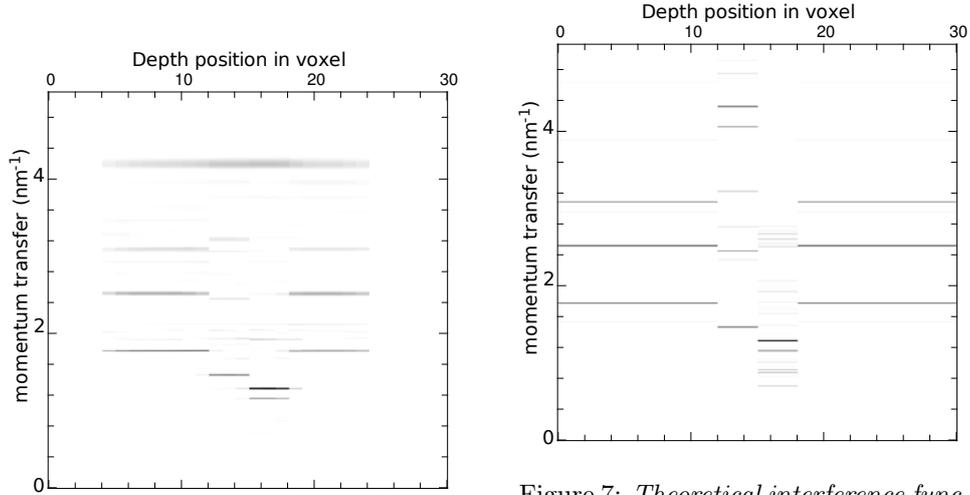
Figure 6: *Crystalline component of estimated interference function map  $\mathbf{f}_{\text{cryst}}^{\text{MAP}}$  by processing data presented in figure 5.*
