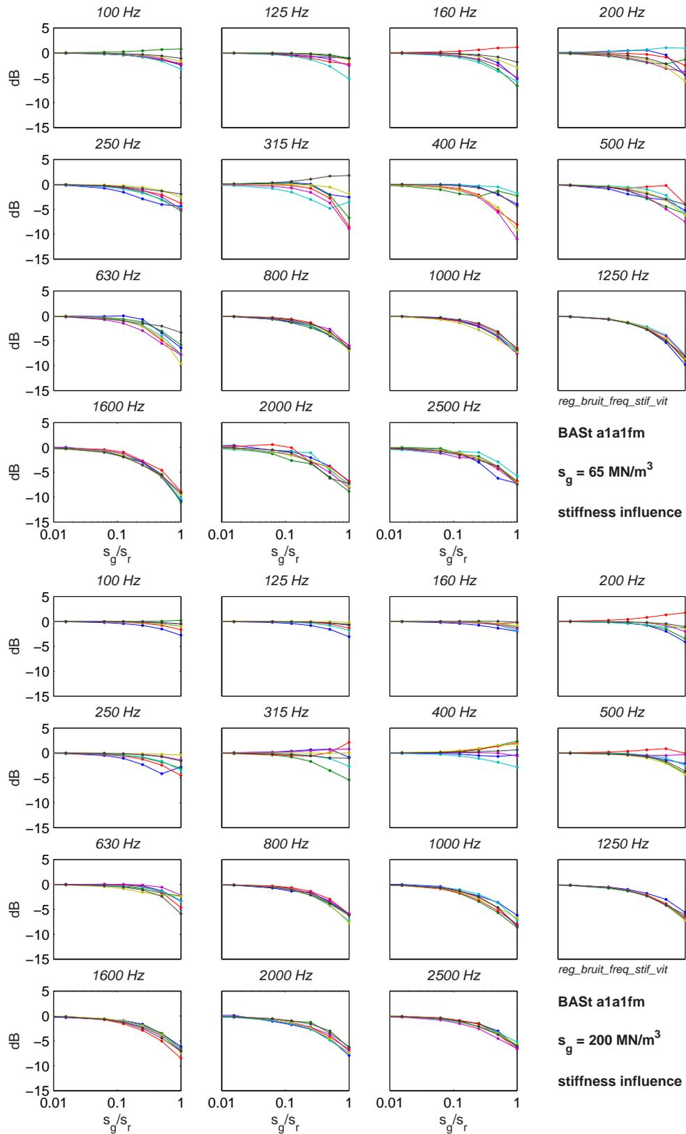
Figure 4.7:  $\Delta L_W = L_W(v, \mathbf{s}_r, f) - L_W(v, \infty, f)$  as function of  $s_g/s_r$ .
