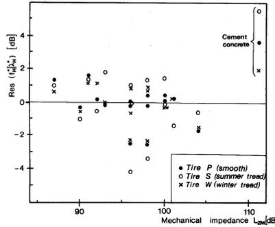
Figure 2.2: The residuals as a function of the mechanical impedance level (dB ref 1N̄s/m) at 2000 Hz [3]
