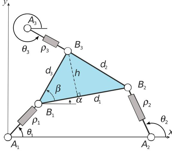
Figure 1: The 3-RPR parallel manipulator under study.
