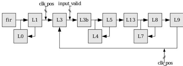
Figure 14: Control flow of the FIR filter
