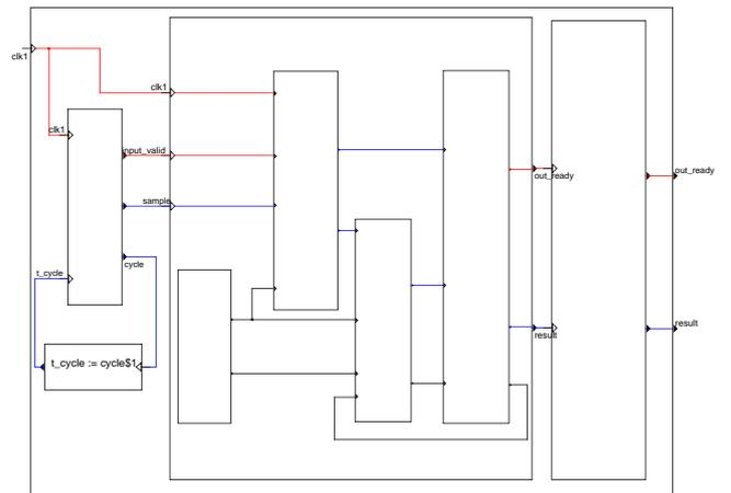
Figure 11: Structure of the FIR filter with testbench
