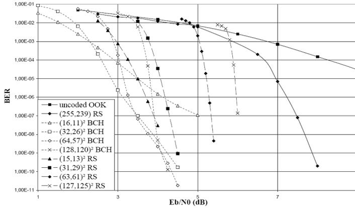
Fig. 1. BTC and (255,239) RS decoding performance
