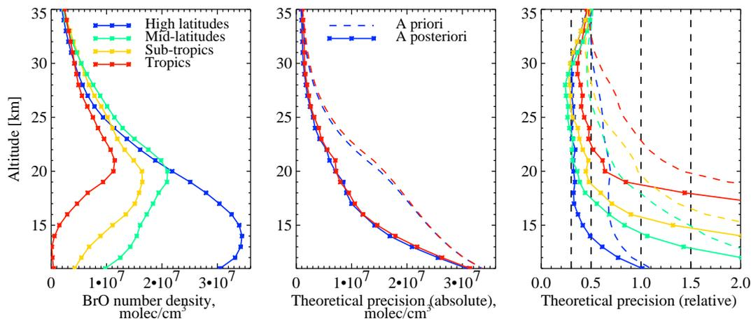
**Fig. 5.** Retrieved vertical profiles of BrO and theoretical precision of the retrieval typical for the IUP Bremen algorithm. Left panel: vertical profiles of BrO typical for high-latitude spring, mid-latitude fall, subtropical summer, and tropical winter seasons. Middle panel: theoretical precisions (solid lines) and a priori constraints (dashed lines) for high-latitude (blue) and tropical (red) retrievals. Right panel: same as in the middle panel but in relative units.
