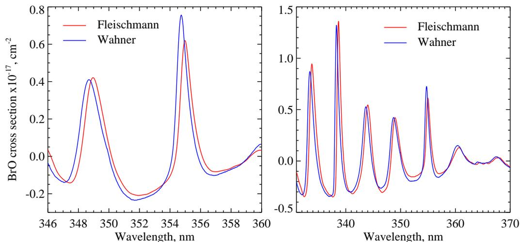
**Fig. 14.** BrO cross section at 223 K according to Fleischmann et al. (2004) shown by the red curve and at 228 K according to Wahner et al. (1988) shown by the blue curve. Left panel: 346–360 nm spectral interval as used in the retrieval of the balloon-borne DOAS measurements. Right panel: 331–370 nm spectral interval as used in the retrieval of the balloon-borne SAOZ measurements.
