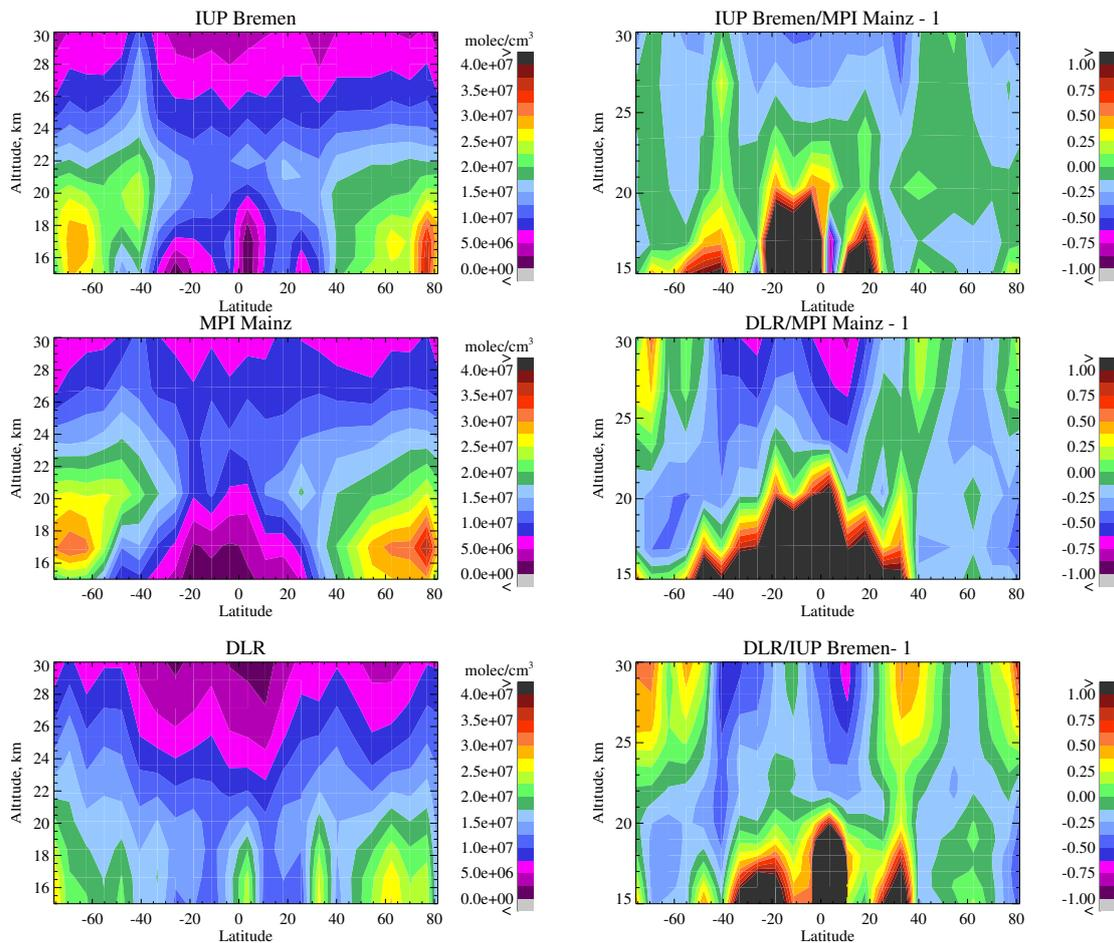
**Fig. 19.** Intercomparison of three SCIAMACHY BrO products for a selected orbit (Orbit 10811, 25 March 2004). Left panels: BrO vertical distributions retrieved from SCIAMACHY limb measurements with different algorithms. Right panels: relative differences in the retrieved BrO profiles.
