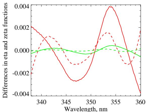
**Fig. 3.** Differential logarithmic eta (red) and zeta (green) functions. The functions are obtained as the spectral residuals remaining when fitting to each other the logarithms of the eta or zeta functions for different positions of the elevation scan mirror. The fit procedure includes the scaling factor and a linear (solid lines) or a cubic (dashed lined) polynomial.
