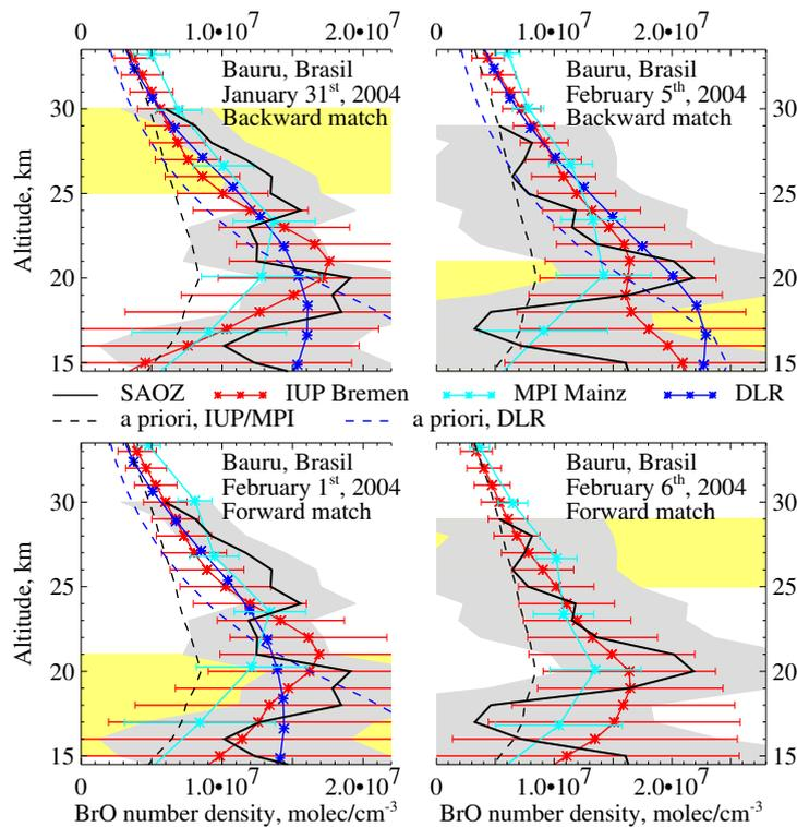
**Fig. 27.** Comparison of BrO vertical distributions retrieved from SCIAMACHY limb measurements using different retrieval algorithms to coinciding balloon-borne SAOZ observations. All balloon launches are in Bauru (tropics). Left panels: 31 January 2004. Right panels: 5 February 2004. Gray shadings depict the uncertainties of SAOZ results ( $1-\sigma$ ). Yellow areas mark vertical ranges where according to trajectory model calculations both instruments probe the same air mass.
