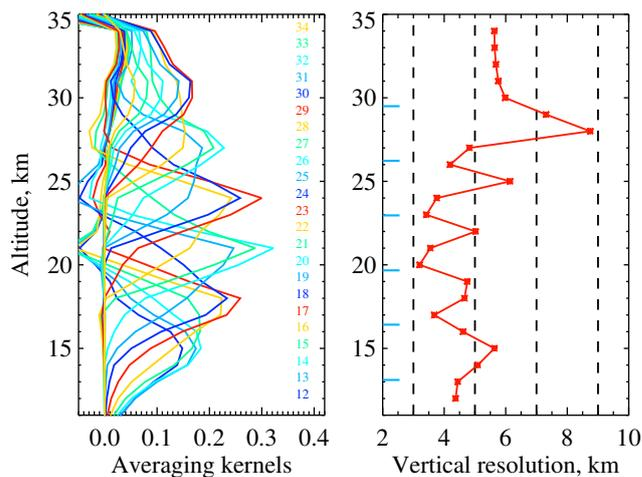
**Fig. 6.** Averaging kernels (left panel) and the vertical resolution (right panel) typical for the IUP Bremen retrieval. The colored numbers on the right-hand side of the averaging kernel plot denote the altitudes which the averaging kernels are calculated for. The thick blue lines in the left-hand side of the vertical resolution plot depict positions of the measurement tangent heights.
