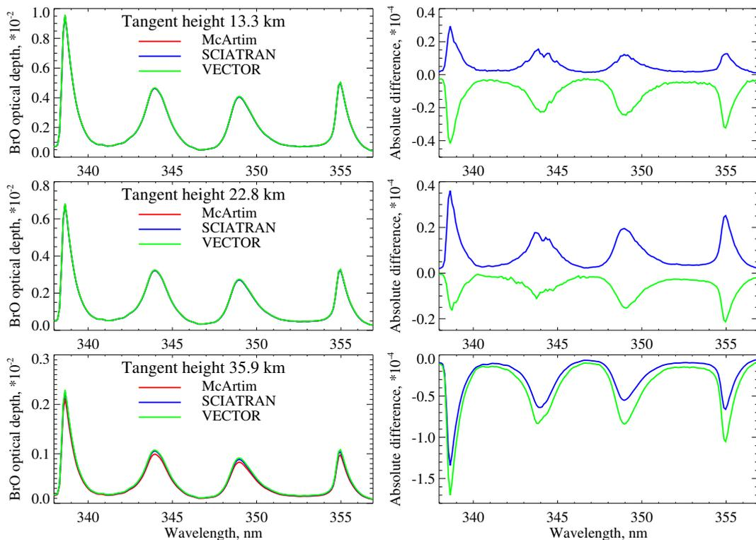
**Fig. 8.** Optical depths of BrO simulated using different radiative transfer models (left panels) and absolute differences in simulated optical depths with respect to McArtim results (right panels) at different tangent heights. The simulations are performed for an observation geometry typical for high-latitude spring stratosphere.
