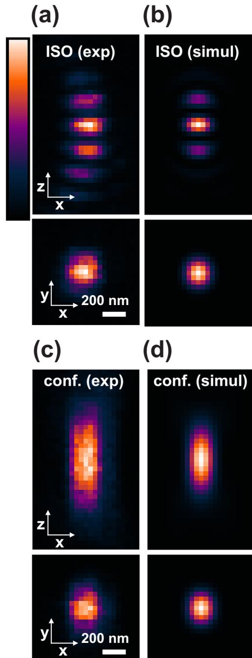
FIG. 6: (Color online).  $xz$  and  $xy$  slices of the 3D image of an isolated 100 nm fluorescent bead. (a) ISO focusing, confocal detection, experimental data, (b) ISO focusing, confocal detection, numerical simulation, (c) out of focus confocal mode, experimental data, (d) confocal mode, numerical simulation.
