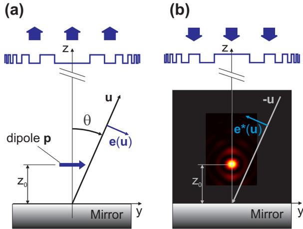
FIG. 2: (Color online). Principles of time-reversal focusing. (a) Radiation of a dipole above a mirror; the blue line depicts the wavefront of the radiated far field. (b) Simulation of the field intensity distribution obtained by illuminating the mirror with a shaped beam whose wave front is the opposite of that of the dipole radiated field.
