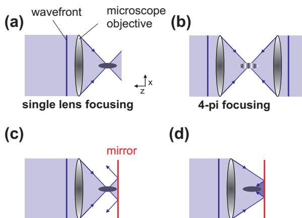
FIG. 1: (Color online). Illumination schemes with (a) a single lens, (b) two lenses facing each other, (c,d) with a single lens and a mirror. Panels (c) and (d) illustrate cases for which the incident and reflected fields do not participate *together* to the spot formation.
