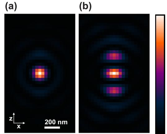
FIG. 4: (Color online). Simulation of the illumination intensity obtained with ISO focusing in water ( $n = 1.33$ ) for  $\lambda = 491$  nm (a) in the ideal case of  $\theta_{\max} = 90^\circ$ , (b) in the case of an objective lens of numerical aperture 1.2, i. e.  $\theta_{\max} = 64^\circ$ . In order to be consistent with the experimental conditions, only the phase of the plane waves was shaped.
