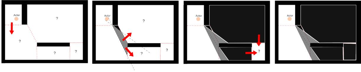
**Figure 5:** Visibility propagation using the cell-and-portal representation. Each visibility prism issued from an edge of a portal is propagated through the portals of the adjacent cells. The process is repeated inside each cell until all cells are explored.
