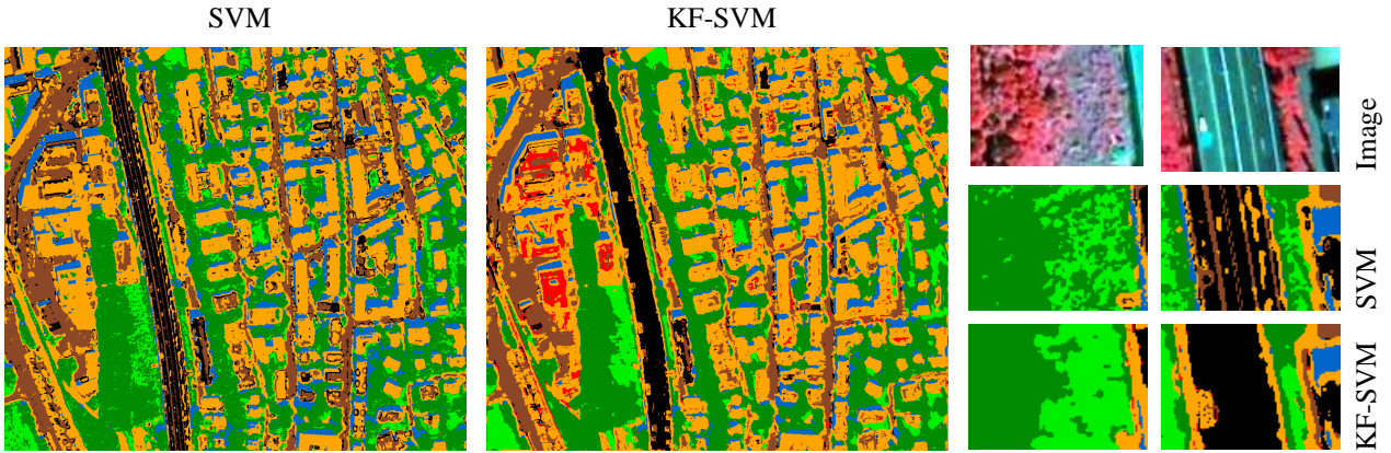
Fig. 3. Classification maps for the SVM and the proposed KF-SVM, for the whole scene and two interesting regions.
