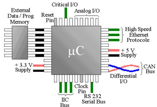
Fig. 2 Potential paths for RFI coupling into micro-controllers.
