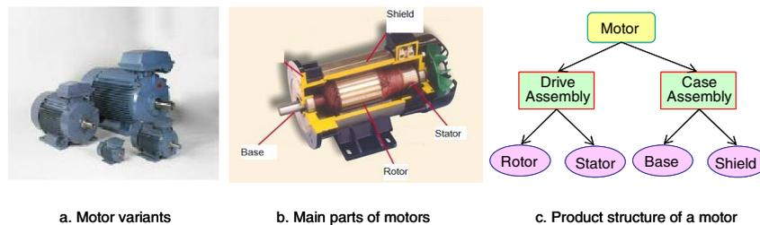
a. Motor variants      b. Main parts of motors      c. Product structure of a motor
