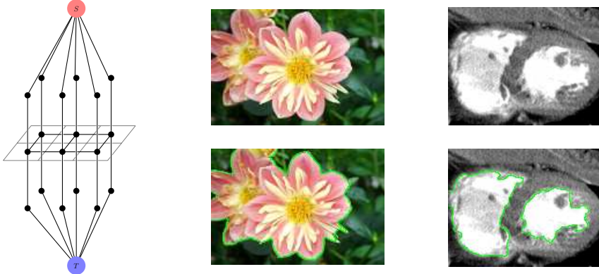
FIG. 4.6. Example of graph construction to incorporate unary terms for unsupervised segmentation. Each node is connected to a source node and sink node through an intermediary node which is weighted to reflect the strength of the positive and negative unary term. This construction is then applied with a simple appearance prior to automatically segment two images.
