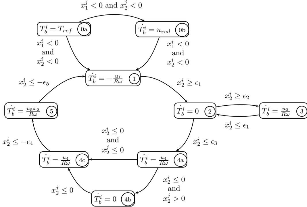
Figure 6: Synchronized ABS regulation logics for the front wheels. The index  $i$  represents the wheel to which the algorithm is applied and  $j$  the opposite wheel.
