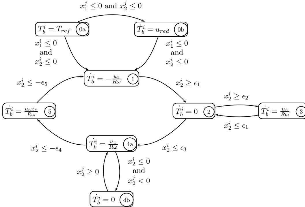
Figure 7: Anti-synchronized ABS regulation logics for the rear wheels. The index  $i$  represents the wheel to which the algorithm is applied and  $j$  the opposite wheel.
